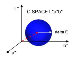
In 3D mode there only is one tolerance for the color space coordinates. The color distance here is calculated from the color space coordinates ( $L^*$   $a^*$   $b^*$ ).
