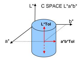
When viewed as a cylinder, the color coordinates (a\* b\*) have their own tolerance (a\*b\*Tol), and the brightness value (L\*) has its own tolerance (L\*Tol). The color distance delta E is calculated from the color coordinates (a\* b\*).
